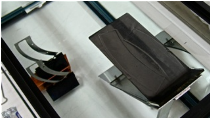
Fig. 8d. Water is added at a controlled slow rate to the lower aquarium until the foil is floating freely. Tare pieces of the floating foil are then carefully removed, and the desired pieces are steered over the frames:
