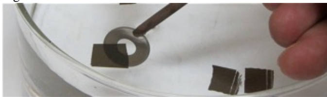
Fig. 9a. Typical pickup sequence for foil onto washer used as a frame. A piece of foil is sequestered, preferably near the edge of the water surface.
