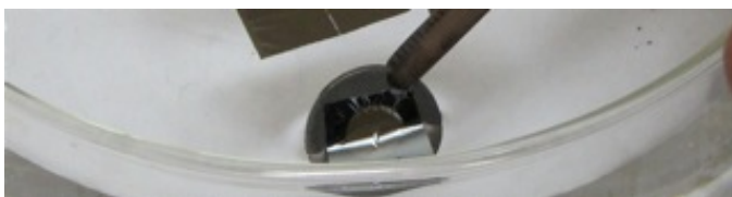
Fig. 9b. The frame is pressed against the piece of foil so that the foil drapes over the aperture to be covered, and then is raised slowly. The foil usually adheres to the exposed surface of the frame.
