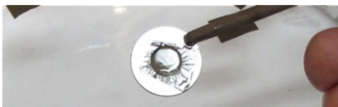
Fig. 9c. When lifted out of the water bath, the foil adheres to the entire perimeter of the washer (frame):
