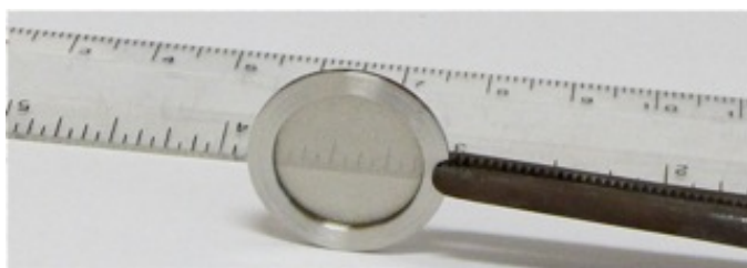
Fig. 5a. Evaporated carbon foil, approximately 5 \mu\text{g}/\text{sq.cm} , on 70 line-per-inch mesh on mounting ring.
