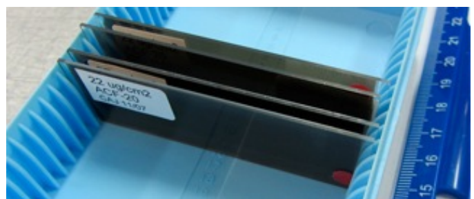
Fig. 1. Evaporated carbon foils (approximately 22 \mu\text{g}/\text{sq.cm} ) on glass substrates 25 mm x 75 mm:
